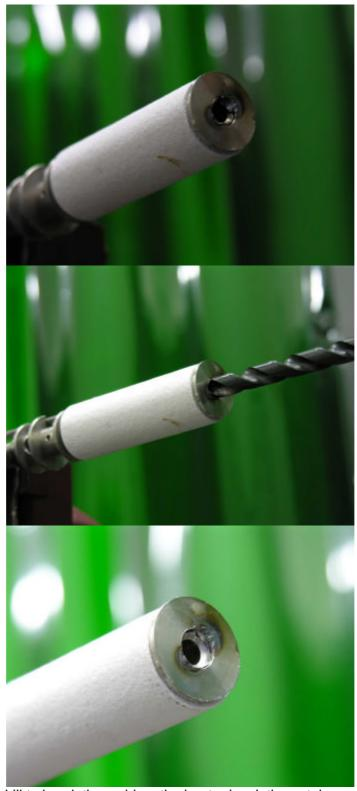
2) Use a 3/8" drill to break the weld on the heater insulation retainer.
