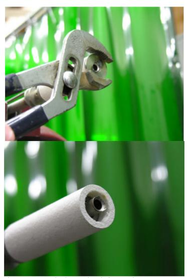
3) Use multi-grips to remove the heater insulation retainer.
