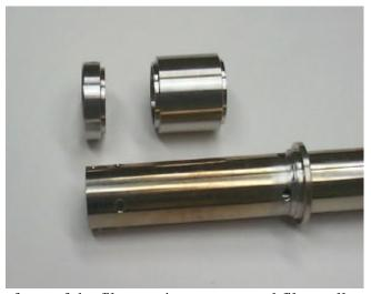
4) Clean the steel surfaces of the filter retainer, spacer and filter collar, especially where the filters make contact with the retainer, spacer and collar.
