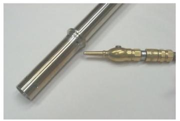
3) Use clean compressed air to dislodge any particulate that may have accumulated inside the filter assembly. If particulate build up is excessive then consider using the 15 micron filters. The finer filters will considerably dampen the response time of the probe.
