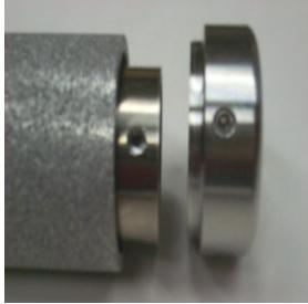
5) Reassemble the filter assembly. The grub screws on the filter retainer should engage the grub screw locking holes at the end of the outer sheath.
