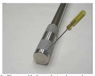
1) To dismantle the filter assembly, loosen the two 4mm grub screws on the end cap.
