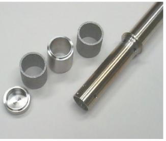
2) Slide the end cap, filters and spacer from the probe.
